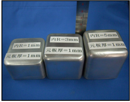
▲Square Cups (t=1.0 mm sheet is used) Punch R 1 mm, R 3 mm, R 5 mm from left side
