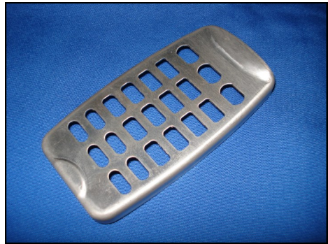
▲Mobile phone cover (t=0.6 mm sheet is used) 48 mm x 82 mm Inner R of outline 2 mm
