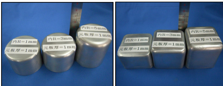
▲Cups (t=1.0 mm sheet is used) Square Cups▲ Punch R 1 mm, R 3 mm, R 5 mm from left side
